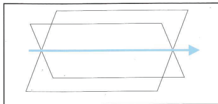
Figure 35: The zone axis is the common crystal direction shared by two planes
